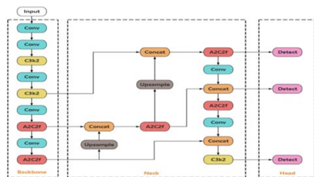
Fig. 1. Architecture diagram of the YOLOv12
